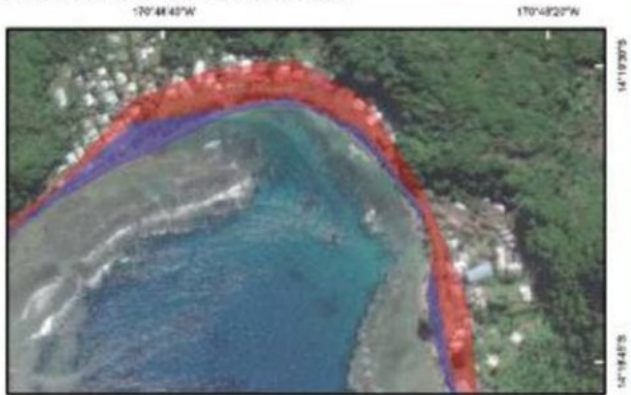
This map shows the simulated flooding for 100-year storm events with (blue) and without (red) coral reefs in Tutuila, American Samoa.
